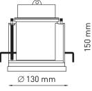
HOLE FOR RECESSING Ø 125 mm
